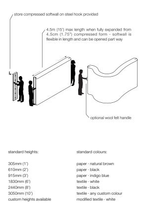
softwall + softblock is a modular, free standing, flexible, partition system at the core of molo's soft collection of paper and textile structures.
