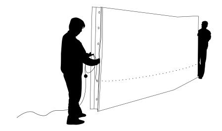
Flexible LED ribbons, designed to go inside the horizontal tunnels of textile softwall + softblock are available from molo in two colour temperatures, a neutral 'daylight white' (4200K) and a 'warm white' (2500K). Only one LED ribbon is needed to create beautifully defused, gradated light within a 1830mm (6') tall softwall.
